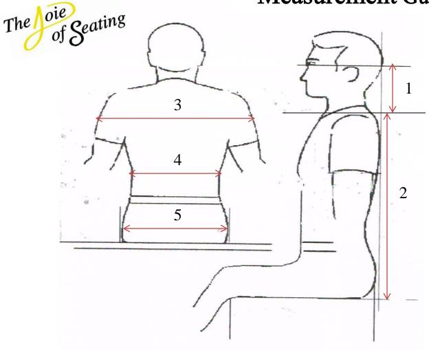
All Measurements should be taken in straight lines with a tape measure, yard stick or stager gauge and photos of these must accompany any seat order.
